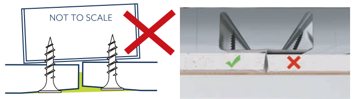
Make sure channel edges are level
